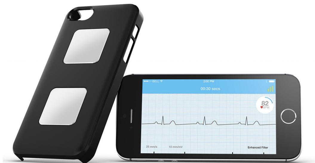
Smartphone monitor and app, with two metal finger pads on reverse and heart rhythm on screen. Reproduced with permission from AliveCor
